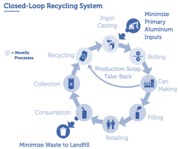
Figure 3: Novelis Closed-Loop Recycling System, Source: Novelis Fact Sheet 14
